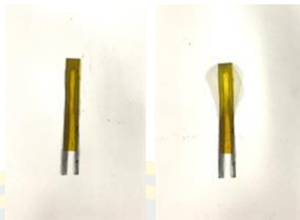
Figure 4-8 The actuator of the PVA/GO/Gly system.
