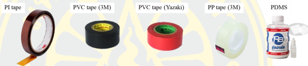
Figure 4-3 Types of polymer layers are: PI PVC (3M) PVC (THAI-YAZAKI) PP (3M) and PDMS.
