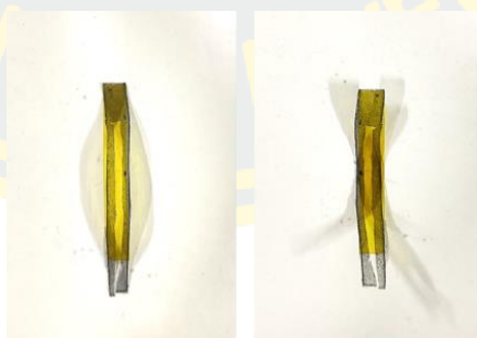
Figure 4-9 The actuator of the PVA/GO/Gly system.
